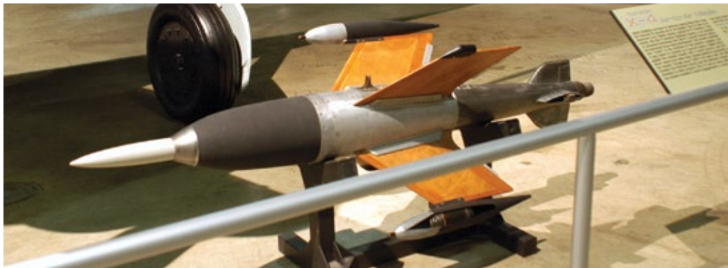
FIGURE 4. GERMAN RUHRSTAHL X-4 WIRE-GUIDED AIR-TO-AIR MISSILE
